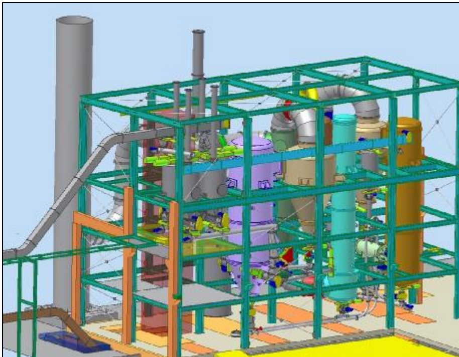
Fig. 3: View of the three-stage fluidized bed system of the CombiPower process
