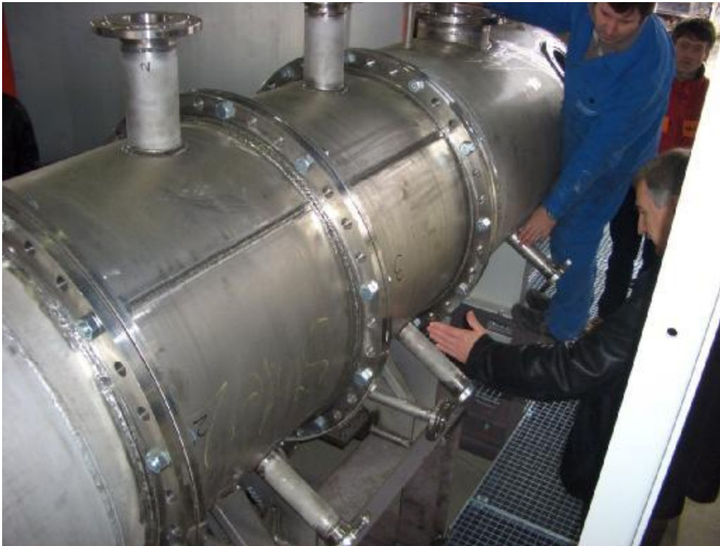
Picture 4: Module 2 + 3 – gassing and gasification zone (LMSV)
